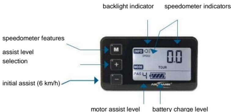
When the system is switched on by turning on the battery, the assist level is automatically set to 2. Using the "+" and "-" keys, the motor assist level can be changed from zero (no assistance) or from 1 to the maximum of 6.
